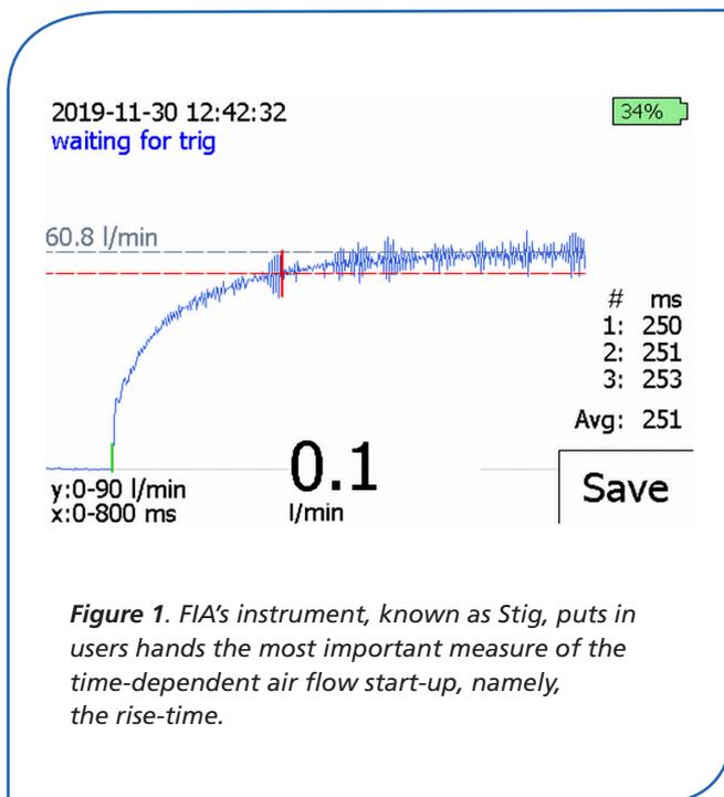
**Figure 1.** FIA's instrument, known as Stig, puts in users hands the most important measure of the time-dependent air flow start-up, namely, the rise-time.
