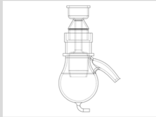
Figure 2. Sampling apparatus for the emitted dose (principle as of reference 2); in the AIM concept the particles have passed through one of FSIs in Figure 1 before being collected in the apparatus.
