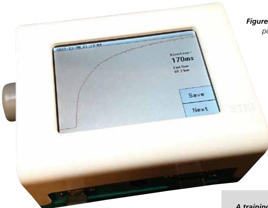
**Figure 1.** FIA's instrument, known as Stig™, puts in users hands the most important measure of the time-dependent air flow start-up, namely, the rise-time.
